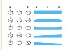
Burner consists of an outer cylinder and 3 inner cylinders. With the manifold adjustment knob, can change the angle of the flame freely and bake goods without any uneven browning.
