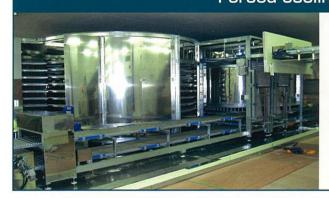
Cooled by air conditioning. Enclosed by panels, cooling quickly within the spiral.
