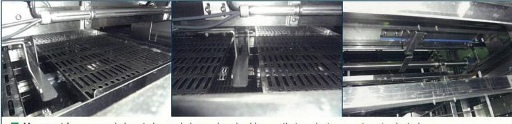
Movement from upper shelves to lower shelves using chucking, so that products are not contaminated.
